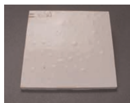
The orthophthalic panel after 15 years.
