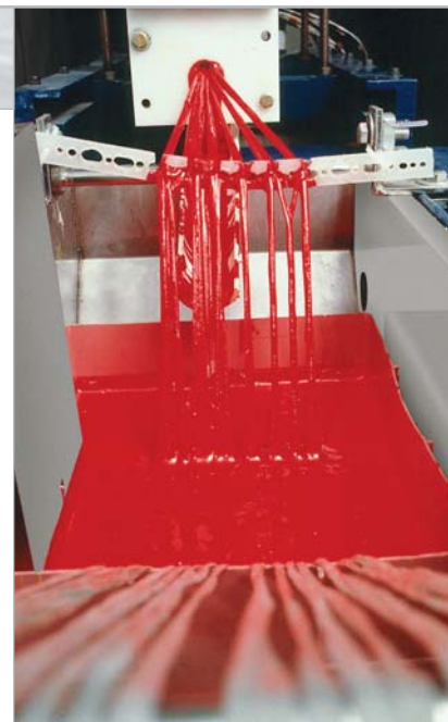
From the resin bath, this pigment-impregnated filament is pulled toward the heated die on our pultrusion machine.
