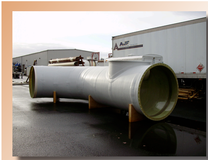
Intel Ducting, 90° elbow with manifold
