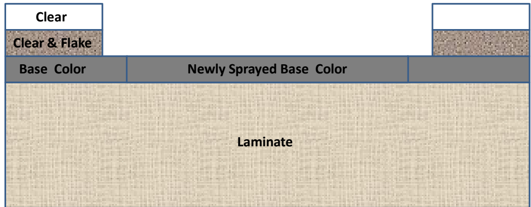
Fig. 7 – Cross Sectional View of Sprayed Area
