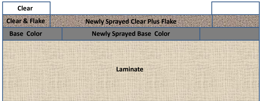
Fig. 9 – Cross Sectional View of Sprayed Area
