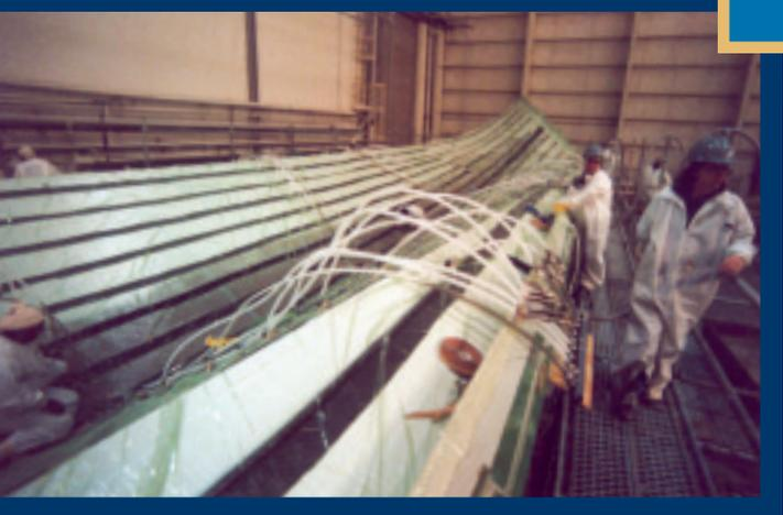
voids on its way. "The infusion process compresses the resin and glass so well you can see right to the core," concludes Gall. The resin-to-glass ratio is reduced to less than 40% of the total laminate volume. The
