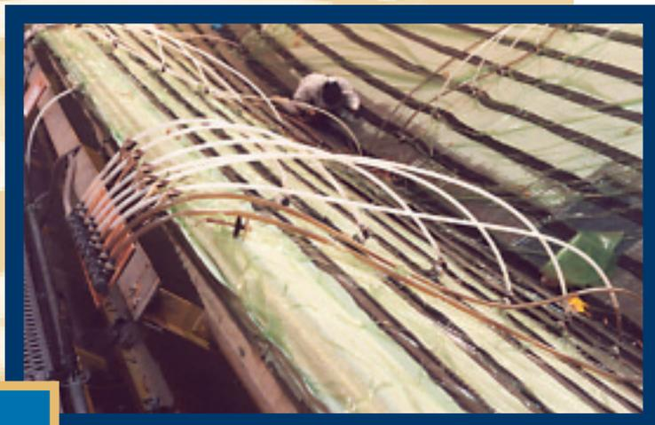
*Clear tubes connect the resin distribution manifold, on the left side, to the resin feeder lines (dark-colored lines) along the hull half.*
