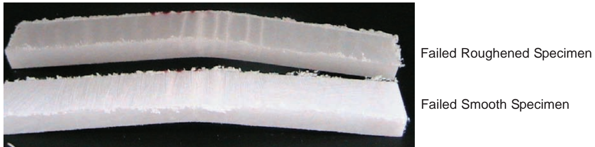
Figure 8: Smooth and Roughened Flexural-Tested Laboratory Specimens
