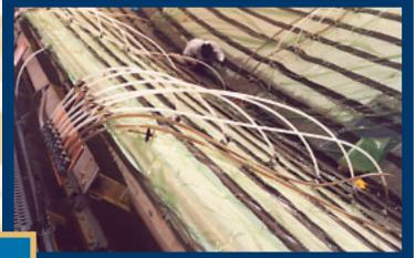
**Clear tubes connect the resin distribution** manifold, on the left side, to the resin feeder lines (dark-colored lines) along the bull balf.
